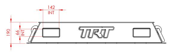
TRT Crane Pads evenly distribute outrigger crane loads. Quality engineering ensures all TRT Crane Pads adhere to the CICA industry standards.
