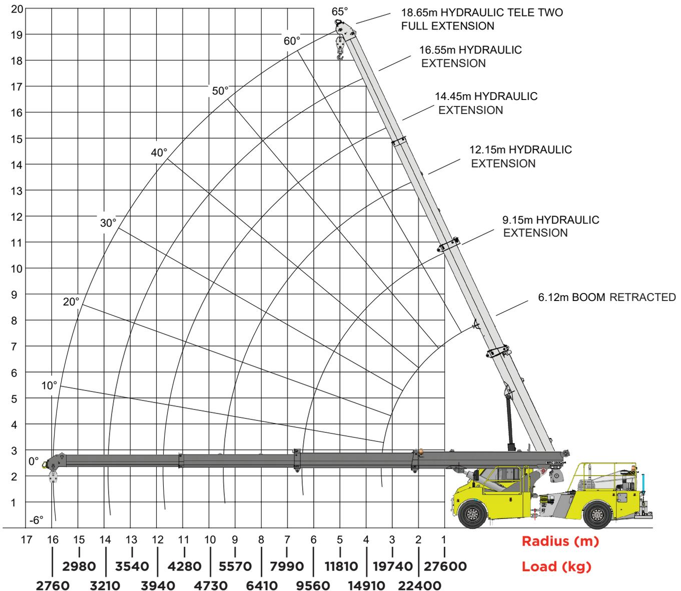
NOTE: Rated capacity values shown are for the stationary chart on the hook.
