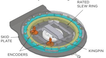
Dual geared encoders at the gooseneck send information to the electronic steering controller when the Prime Mover turns to optimise the steering angle.
